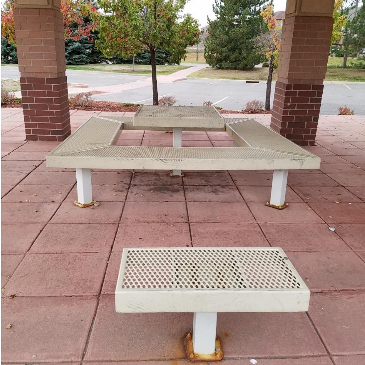
Figure 19. This picnic table in the Boulder suburbs requires one to be able-bodied enough to either step over the bench or swing one's legs over the bench to sit facing the table, which could be an issue for those with problems in the lower back, hips or legs. (Photos: PJ Dellenbaugh)
